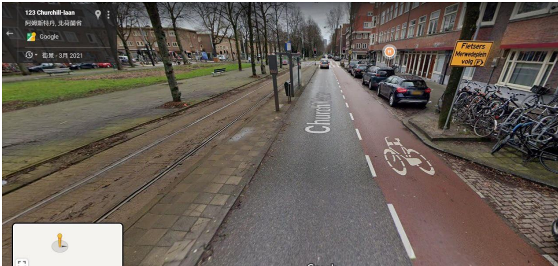
▲ A non-physically separated lane for slow-moving vehicles in the Netherlands. 68
