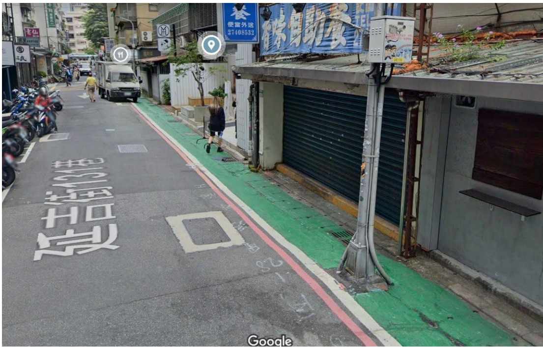
▲ Passage difficulty due to insufficient width caused by streetlamp 46
