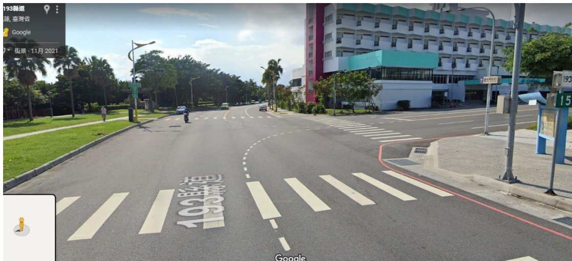
▲ Crossings without recession and no railings to prevent pedestrians in a rush from crossing roads in sections without crossings. 51
